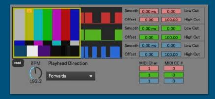
Smoothing control makes value changes less sharp Offset allows for a constant value to be added or subtracted from the output Low and High Cut controls allow for fine-tuning the output range
